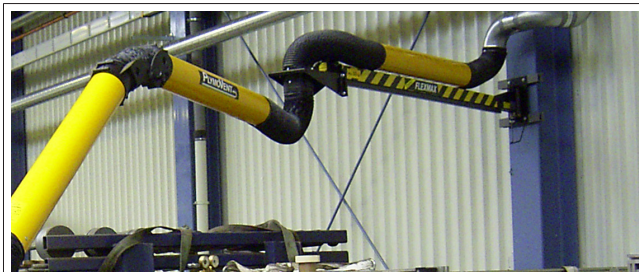
The FlexMax can be mounted in areas with a low ceiling (min. mounting height 2 m / 6.6 ft)
